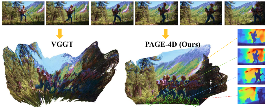
Fig. 1: PAGE-4D takes a sequence of RGB images depicting a dynamic scene as input and simultaneously predicts the corresponding camera parameters and 3D geometry information—all within a fraction of a second. Compared to VGGT, PAGE-4D produces denser and more accurate point cloud reconstructions with better depth estimation quality. (Best viewed in PDF.)
